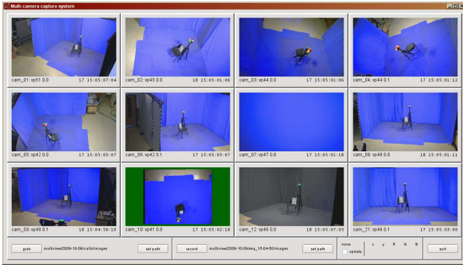
Figure 3: A simple GUI client controlling 12 camera channels.
