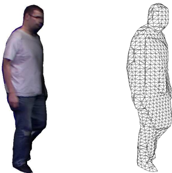
Figure 5: Reconstructed mesh with simple texturing and wireframe of the mesh.
