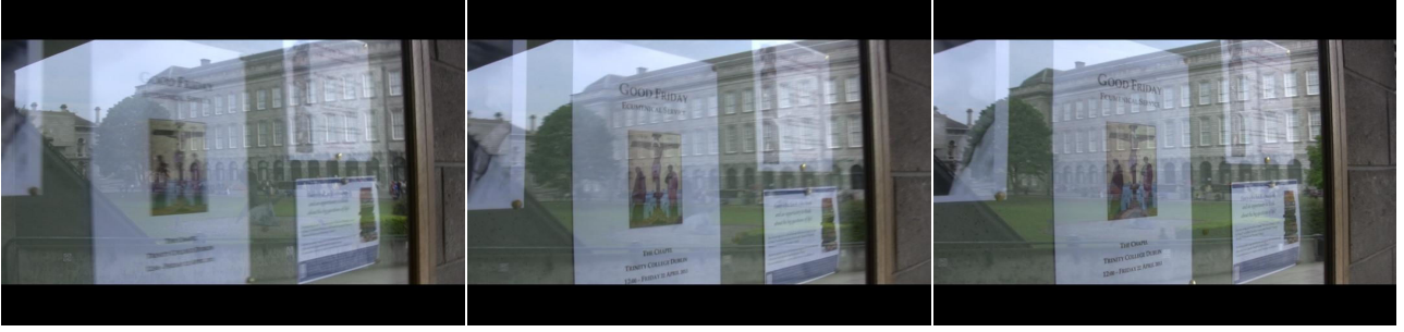
Figure 1: From Left; Frames 5,17,25 from a sequence containing reflection of a building superimposed on paper posters. In this sequence the building is moving to the left while the posters are moving to the right. This generates two motion vectors per pel.
