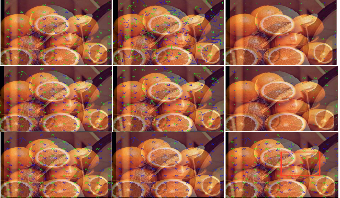
Figure 4: Multiple motions for frame 11 (top row) and frame 12 (second row) as estimated by, From left; BIMS, FTRANS and OPTIC. Green and blue vectors represent the estimated motions of Lenna and Oranges respectively. Motion estimations of BIMS for the two frames are v_{1n} = (-2, -3) , v_{2n} = (2, 3) , v_{1_{n+1}} = (2, 3) and v_{2_{n+1}} = (-2, -3) respectively. Motions shown in the figure are scaled by a factor of 5 for illustration clarity. BIMS generated motion-layer labeling that is temporally consistent despite the strong motion discontinuities in the examined sequence. However, FTRANS and OPTIC failed to handle the strong motion discontinuities. Last Row: Examining effect of terms (on frame 12). From Left: Turning OFF the temporal consistency term from BIMS generates motion-layer labeling that is temporally inconsistent with frame 11; Turning OFF the layer structural independence term from BIMS generates one motion per examined site; Turning OFF the motion spatial smoothness term from BIMS generates motion-layer labeling that is spatially inconsistent (see the red box).
