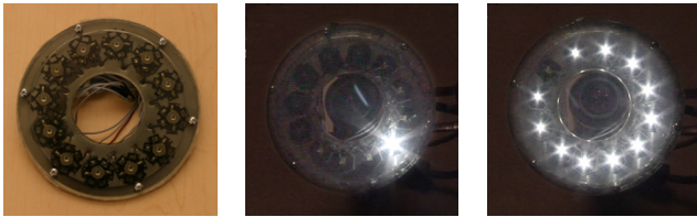
Figure 2: (left) The LED ring, (center) a single-LED pattern, (right) a gradient LED pattern.
