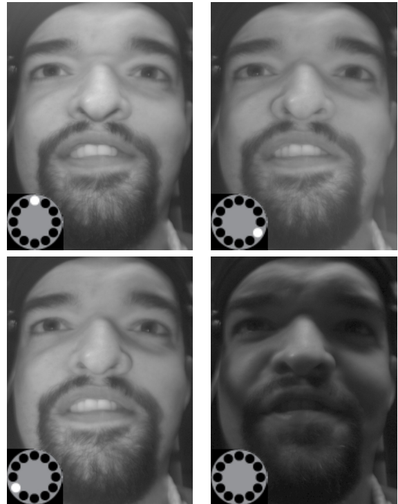
Figure 3: Four time-multiplexed illumination conditions using single visible LEDs, showing three lighting directions and an image of only the ambient light in the environment
