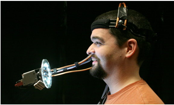
Figure 1: Head-mounted camera and LED light ring
