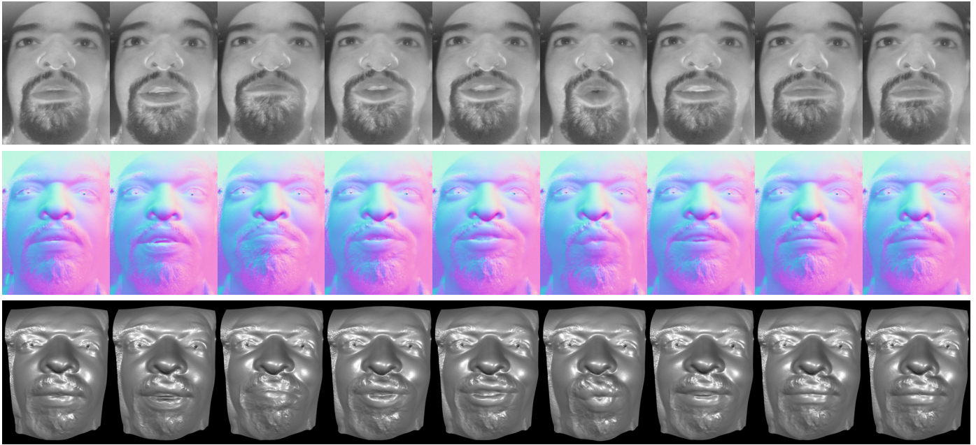
Figure 8: Results showing every 18th frame from a performance captured under single LED illumination. (row 1) Surface albedo recovered using photometric stereo, (row 2) surface normals with XYZ encoded as RGB, (row 3) integrated surface geometry.
