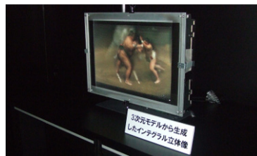
Figure 13: 3D display using integral photography
