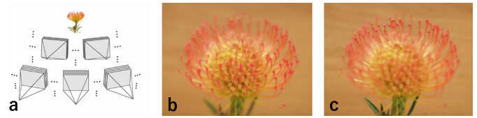
Figure 1: We perform focus bracketing from multiple viewpoints and train a network using the obtained photographs (a). We synthesize from an unknown camera with different focus distances (b) and (c).
