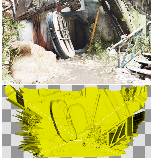
Figure 2: Top: Virtual content rendered in Unreal Engine. Bottom: Reprojection geometry generated in real time from the content’s depth map.
